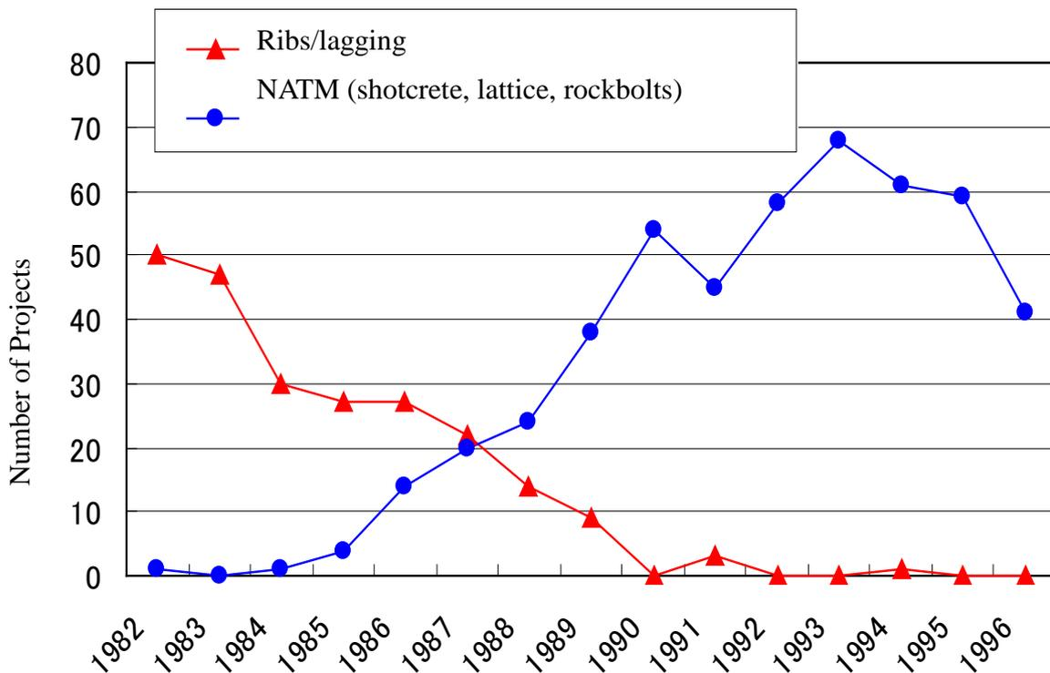
**Figure 4 Data Documenting the Change in U.S. Road Tunnel Support Methods Between 1980 and 2000 (data from FHWA)**
