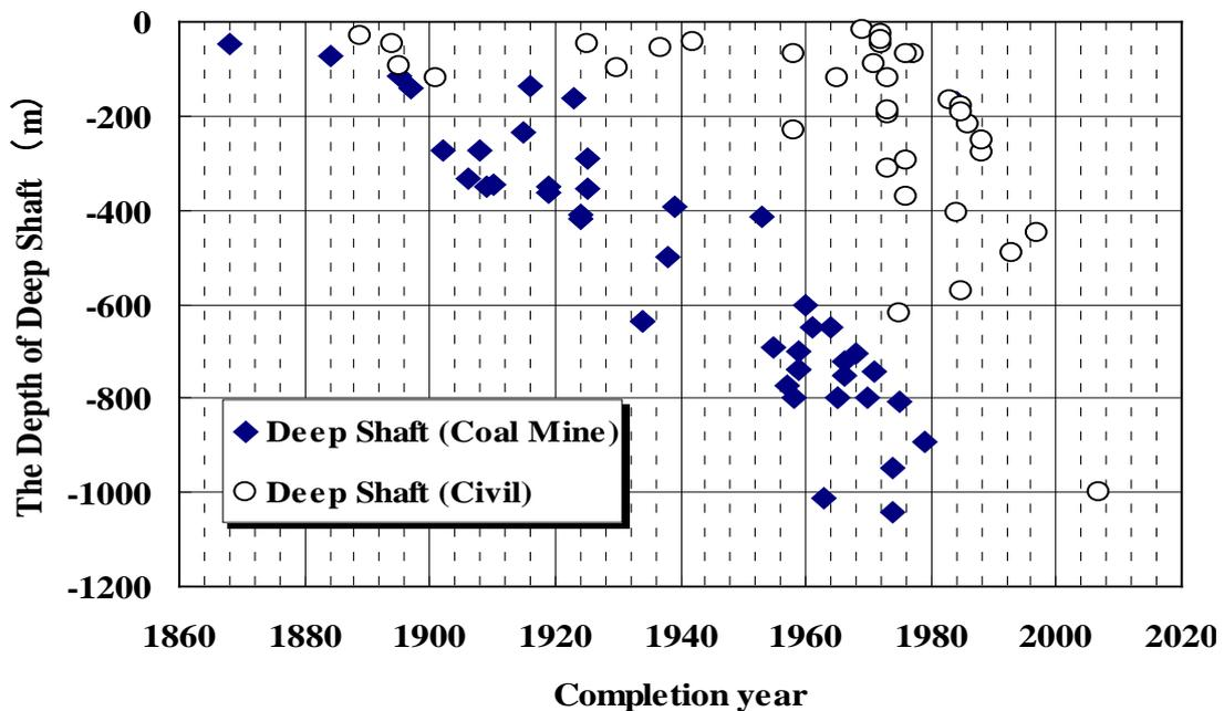
**Figure 2. U.S. Data on Depths of Coal and Civil Deep Shafts 1860 – 2010**
