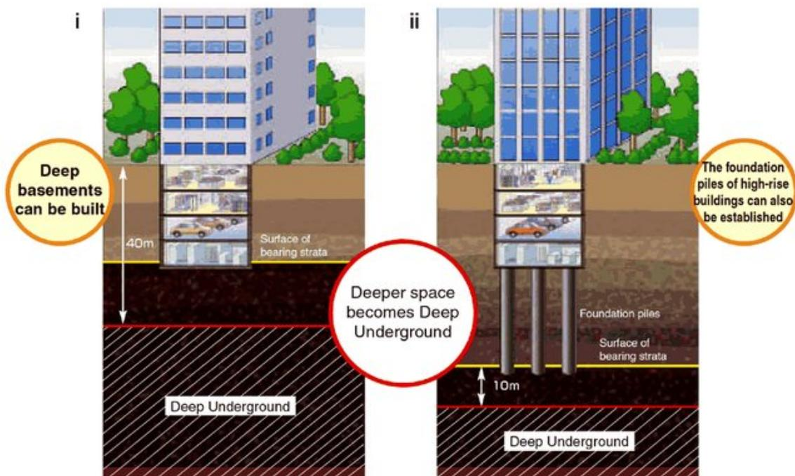
**Figure 3. Schematic of Impacts of the 2001 Deep Underground Utilization Law in Japan (Li, 2013)**
