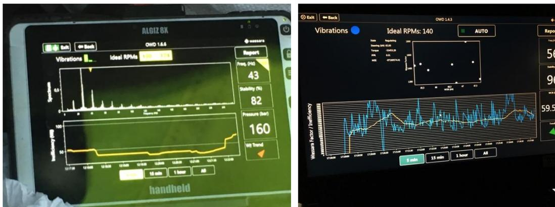
Figure 2. LKAB Wassara OWD® stand-alone unit in open-loop mode and its closed-loop counterpart in auto mode continuously regulating rig parameters.
