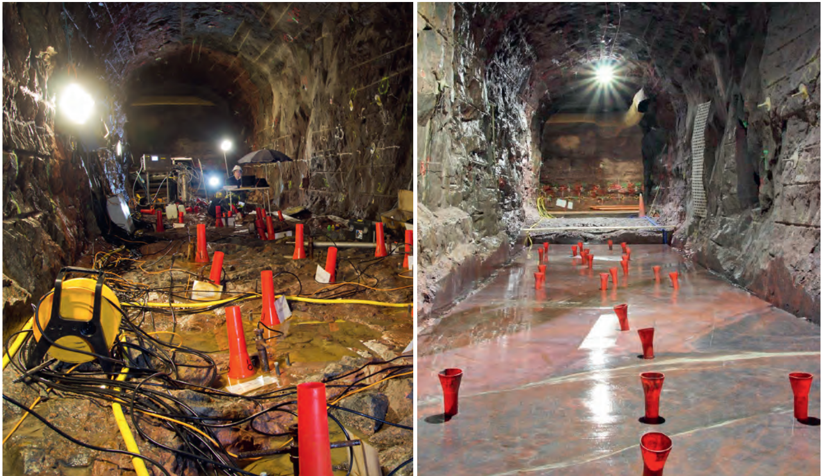
Investigations of excavation-damaged zone in tunnel floor at Äspö HRL. Comparison of hydraulic conditions after blasting and wire cutting respectively. Photos: SKB and Rickard Enér.
