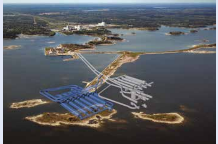
Diagrams showing the arrangement of the planned Spent Fuel Repository (SFR) at the Forsmark nuclear power plant, in Sweden
