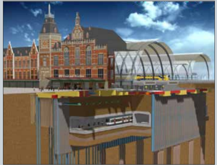
Visualisation of the North/South metro line works in Amsterdam
